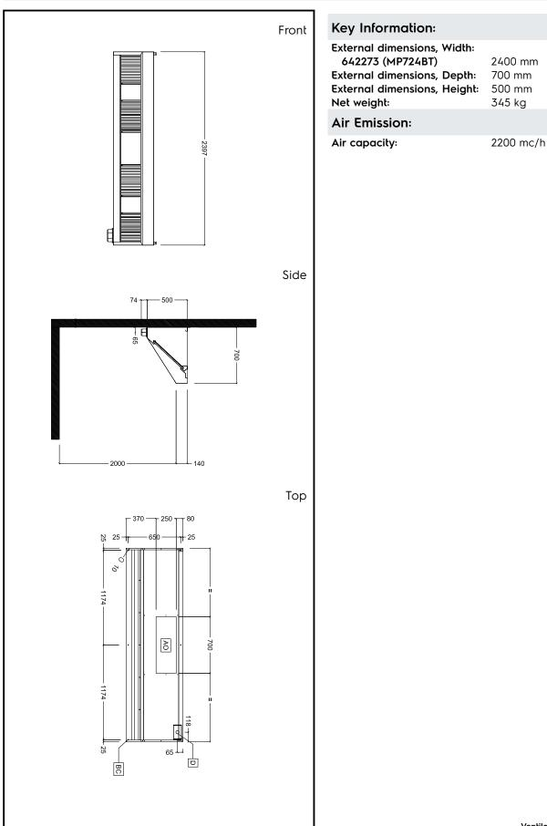
Ventilation Equipment 430 S/S Wall Hood+Filters 2400X700mm
